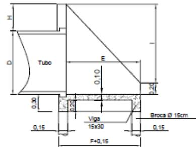
CORTE AA DETALHE DE MURO DE ALA
