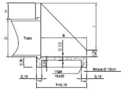
CORTE AA DETALHE DE MURO DE ALA
