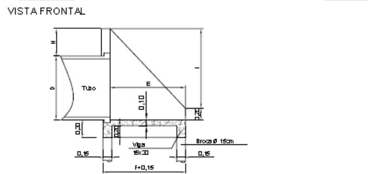
CORTE AA      DETALHE DE MURO DE ALA
